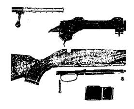
care should be used in this operation so that the stock finish is not chipped. The action should be removed from the stock if the rifle has been in a heavy rain or other adverse conditions so that metal parts covered by the stock can be dried off. A coating of wax or grease should then be applied to the underside of the barrel and action before reassembly. Reverse this procedure to assemble action to stock.
