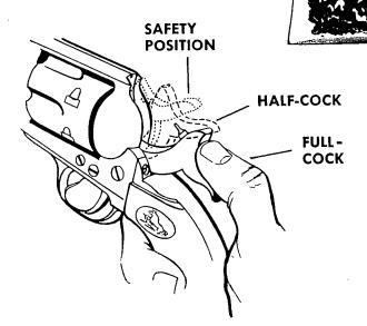
FULL-COCK—with the hammer all the way back and the revolver ready to fire.
